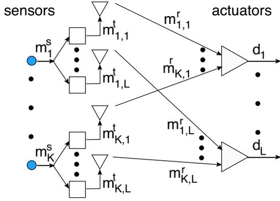
**Figure 1: A schematic of the communications pathways in the WSAN model. The  $k^{\text{th}}$  sensor makes a noisy reading  $m_k^s$ . The quantized measurement  $m_{k,l}^t$  with  $B_{k,l}$  bits of precision is sent to the actuator  $l^{\text{th}}$  actuator. After incurring bit errors in the wireless channel, the measurements  $m_{k,l}^r$  are received by the actuator and used to form the approximate actuation coefficient  $\hat{d}_l$ .**
